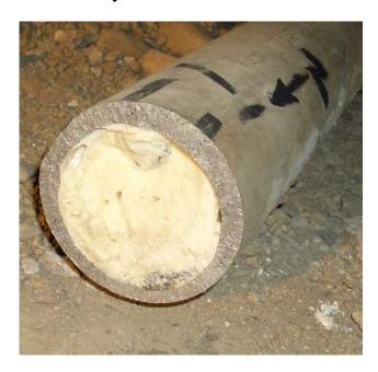
Autopour foam stabilizes pipes and reduces the potential for spread of contamination during size reduction activities.
